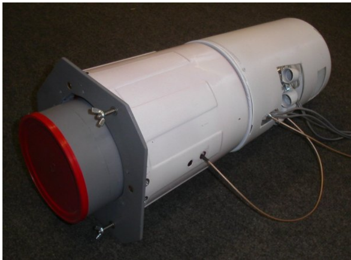
Figure 6 Complete Head Amplifiers and cylindrical feed assembly
