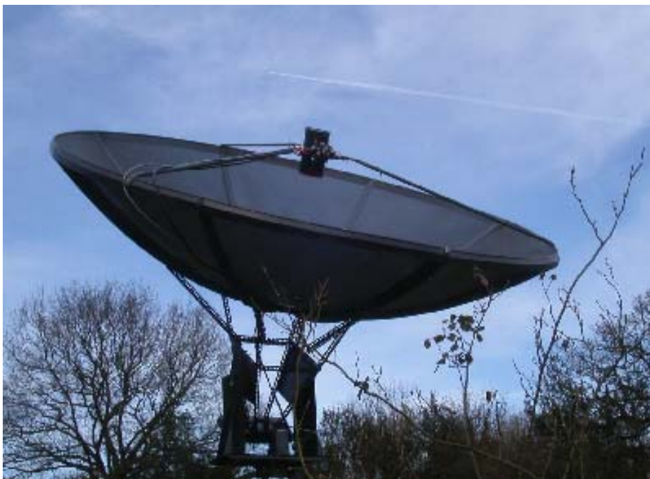
Figure 2 - 3m' Dish with 1420MHz Cylindrical Waveguide Feed
