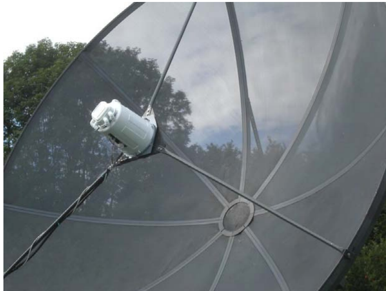
Figure 1 3m diameter F.28 dish with cylindrical waveguide feed
